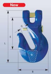
The **Shortening Hook TWN1827/1** according to DIN 5692 makes the lifting of loads safer. The new shape of the shortening Hooks TWN 1827/1 offer you much more safety than with conventional shortening hooks. The extra wide chain attachment enables us toguarantee you an especially firm seating of the inserted chain link and it is also protected from damage at the same time. The locking pin prevents an accidental loosening of the sling chain.
